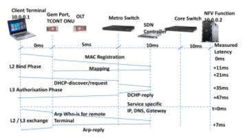
Fig. 3 Service Registration on SDN/NFV testbed
