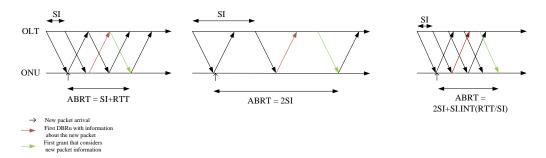
Fig. 3. Assured Bandwidth Restoration Time for GIANT.
