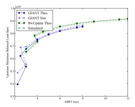
Fig. 7. Theoretical and simulated maximum balanced load vs. ABRT.
