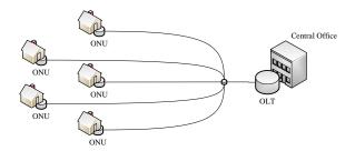
Fig. 1. Typical Fibre To The Home architecture
