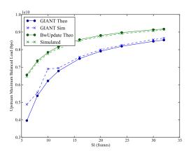
Fig. 6. Theoretical and simulated maximum balanced load vs. service interval.
